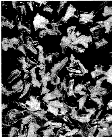
Figure 1: Photomicrograph of silicic glass shards formed from broken bubbles. White zones within some shards are microvesicular frothy areas (magnified 60 x).
