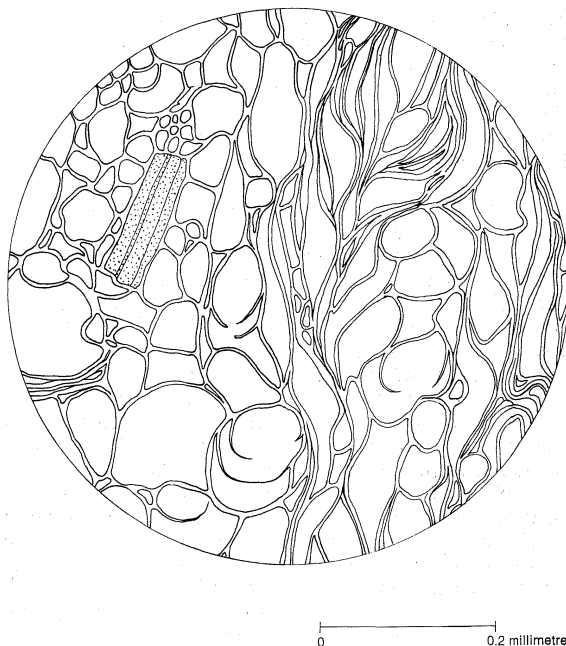
Figure 2: Vesicular structure of silicic pumice as seen under microscope.
